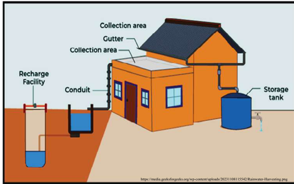
Fig 22: Components of a Rainwater Harvesting set-up
